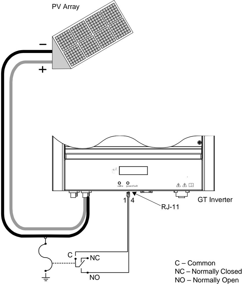
Figure 2 Connections (PV Negative Ground Configuration Shown)
